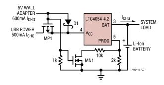
Figure 7. Combining Wall Adapter and USB Power
