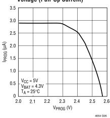
PROG Pin Current vs PROG Pin Voltage (Clamp Current)
