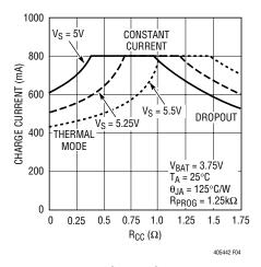
Figure 4. Charge Current vs R<sub>CC</sub>
